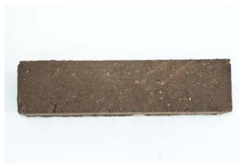
Figure 6: Test sample of a hardened backfilling product
