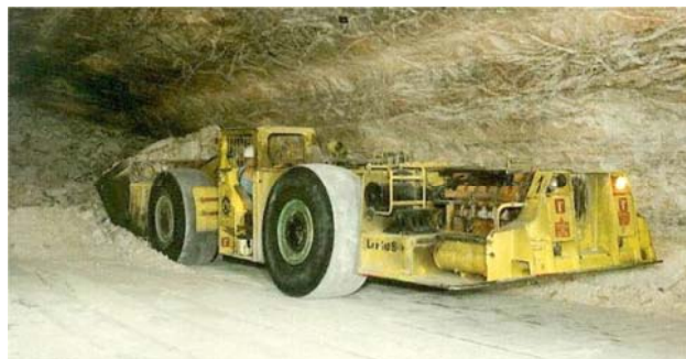
Figure 2: Backfilling of a mining site with bulk goods
