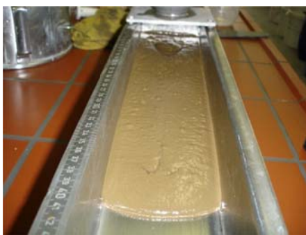
Figure 5: Determination of the flow extent of a viscous slurry mixture
