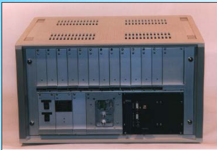
Demodulation unit with integrated transient recorder
