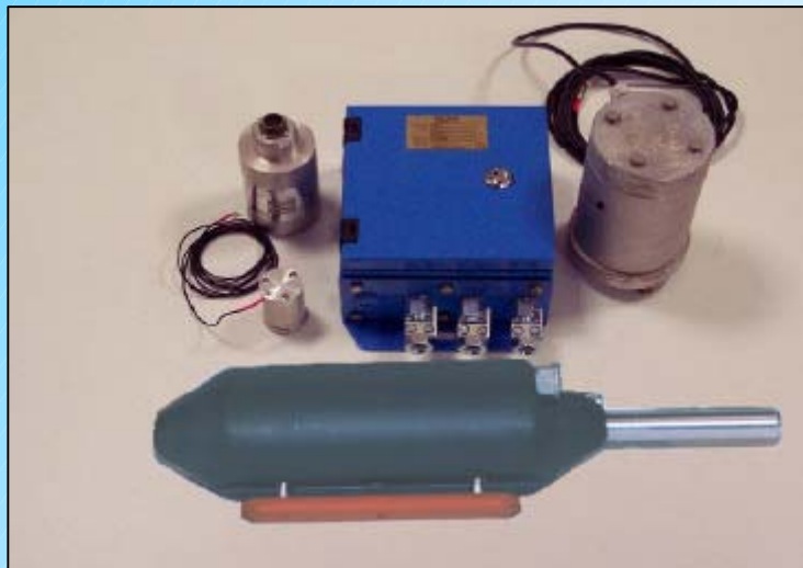
PFM-modulator and various types of seismometers
