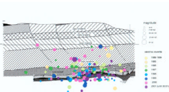
Figure 6: Cross section through the mining field and depth distribution of the seismic events
