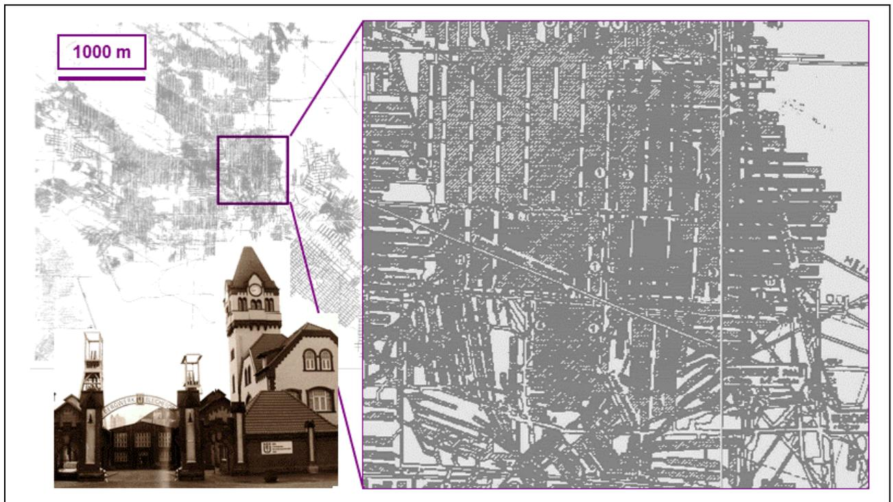
*Figure 3: Area of total pillar re-mining in the central field of the mine Bleicherode as a detail figure on the right side and in the principal mine layout on the left side.*
