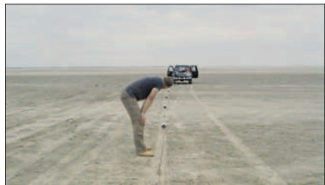
Figure 3 OhmMapper in the field behind the investigation truck.
