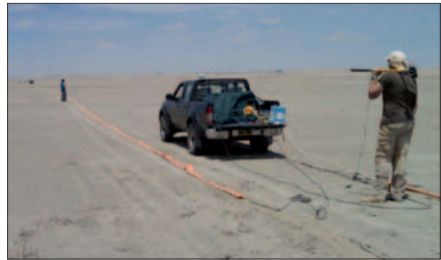
Figure 1 Investigation car with the registration units, the GPS unit and the Landstreamer.
