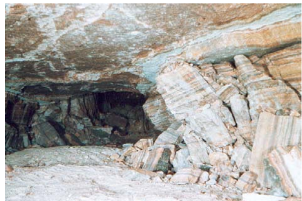
Figure 1: Destruction of pillars in the abandoned carnallite mining field.
