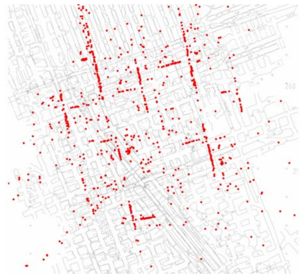
Figure 7. Distribution of recorded micro-seismic events in the mixed salt mining field.
