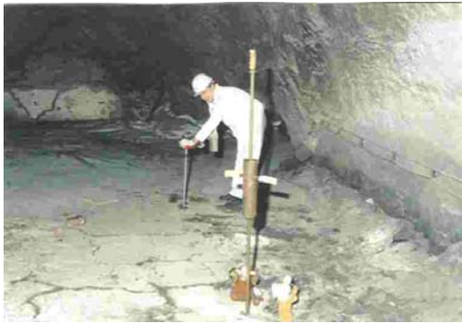
Figure 6. Measurements of the shearing strength and drop-penetration tests in hardened hydraulic backfilling
