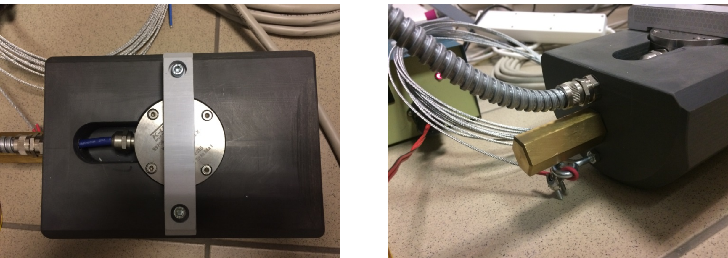
Figure 2: Seismometer L-10B/Ex with borehole probe
